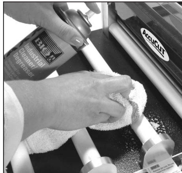
Spray white rollers with Bio-T® Foamaxx Cleaner (Item TSC1040), or another all-purpose cleaner, then wipe clean.
