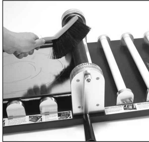
Wipe top roller with a clean, dry rag—or brush away small scraps.
