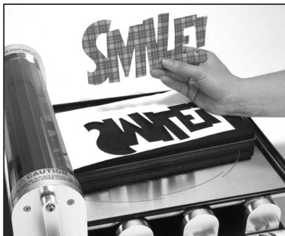
Figure 3: Placing paper with pattern side down is especially important when cutting letters or words, so the pattern will be on the correct side.
